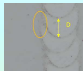
Fig. 6 shows consecutive overlapped laser spots
