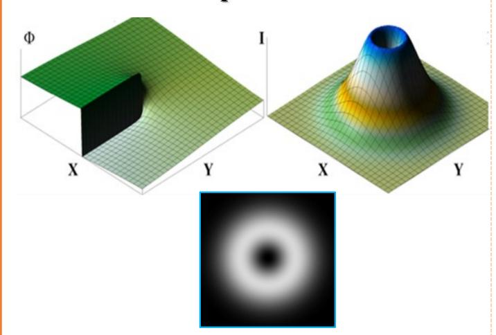
Above are shown phase and intensity distributions of an optical vortex with topological charge = 1.
