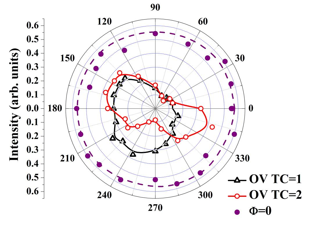
**Polar plot:** Same as Graph (d) above, however for phase OVs of topological charges TC=1 and TC=2 generated by a liquid crystal on silicon based spatial light modulator used as an unknown polarization influencing element.
