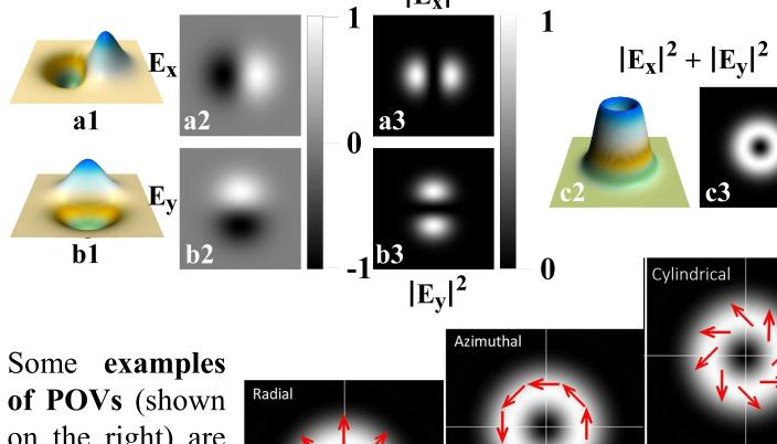
Some examples on the right) are radially, azimuthally, cylindrical polarized beams.
