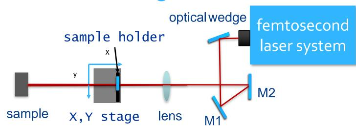
A modified Z-scan method was applied to synthesized glasses, enabling simultaneous evaluation of the nonlinear refractive index ( $n_2$ ) and the absorption coefficient ( $\beta$ ). The technique relies on the conversion of phase to amplitude distortion during beam propagation and provides higher accuracy and reliability compared to the classical setup.
