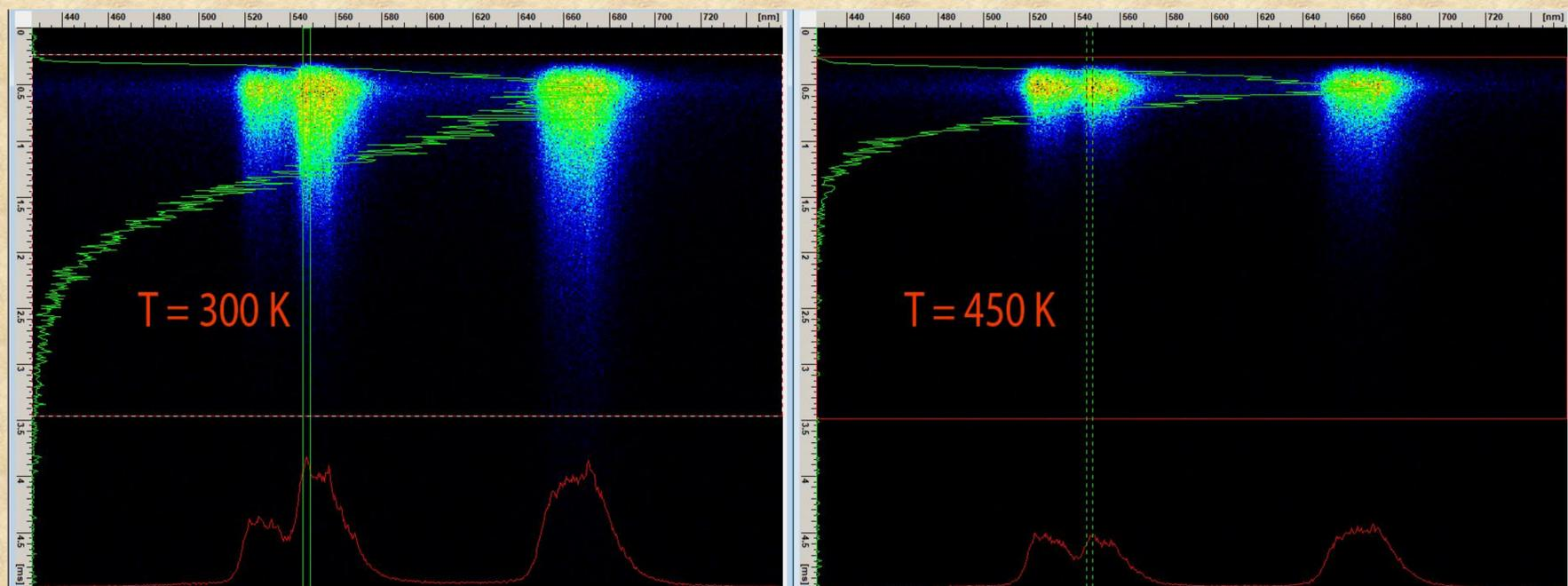
Streak images of  $Gd_2O_3:Er^{3+},Yb^{3+}$  excited at 980 nm, at different temperatures. Images are presented in pseudocolor where different colors correspond to different intensities. Vertical axis corresponds to time, here it is 5 ms from the start to the end of streak image. Horizontal axis corresponds to wavelengths of optical emission.
