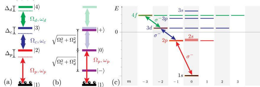
Figure 2: (a) The light-matter coupling scheme in the bare-state basis. (b) Dressed states of the SQD with  $\Delta_p = \Delta_c = \Delta_d = 0$ . (c) The schematic depiction of three laser fields and few lowest energy levels for the SQD with  $R = 81.76$  nm.
