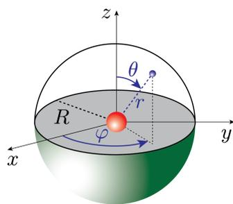
Figure 1: The schematic depiction of the SQD with the on-center hydrogen impurity.
