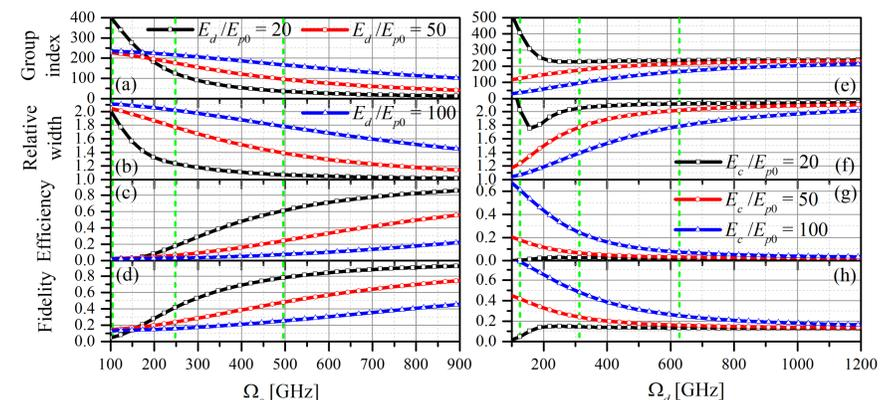
Figure 5: The output pulse parameters as functions of the Rabi frequency of the (a-d) control field and (e-h) additional control field. The values of  $\Omega_c$  and  $\Omega_d$  used in the previous figures are given in green dashed lines.
