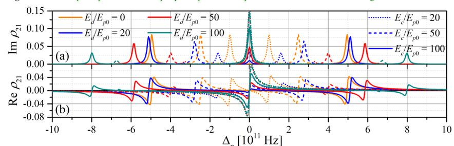
Figure 4: The (a) absorption and (b) dispersion curve for the four-level cascade system with  $\Delta_c = \Delta_d = 0$  and several values of the strength of the control fields.
