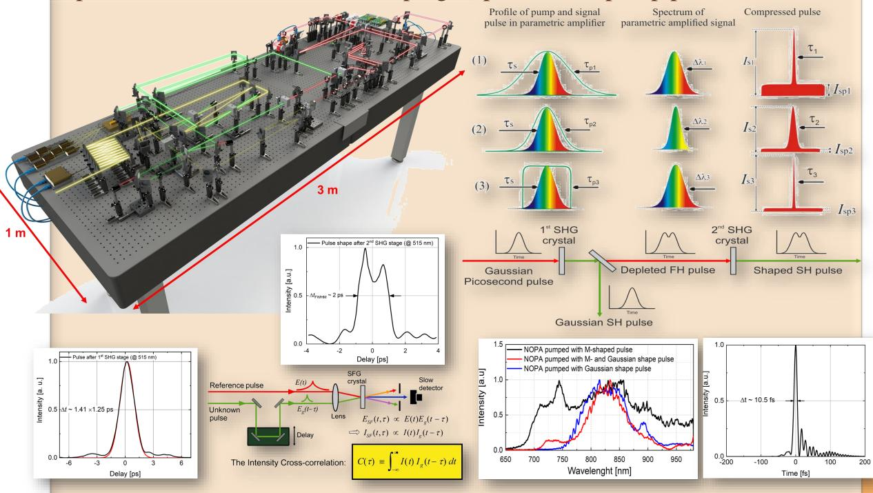
The pulsewidth after compression reaches 12 - 15 fs, and the output energy is mainly limited by the number and power of laser diodes used for pumping, providing the output peak power of the laser system from 0.1 to 1TW. The experimental scheme is assembled on an optical table measuring 1 x 3  $m^2$ , all components used are commercially available, and the repeatability is confirmed by student interns.
