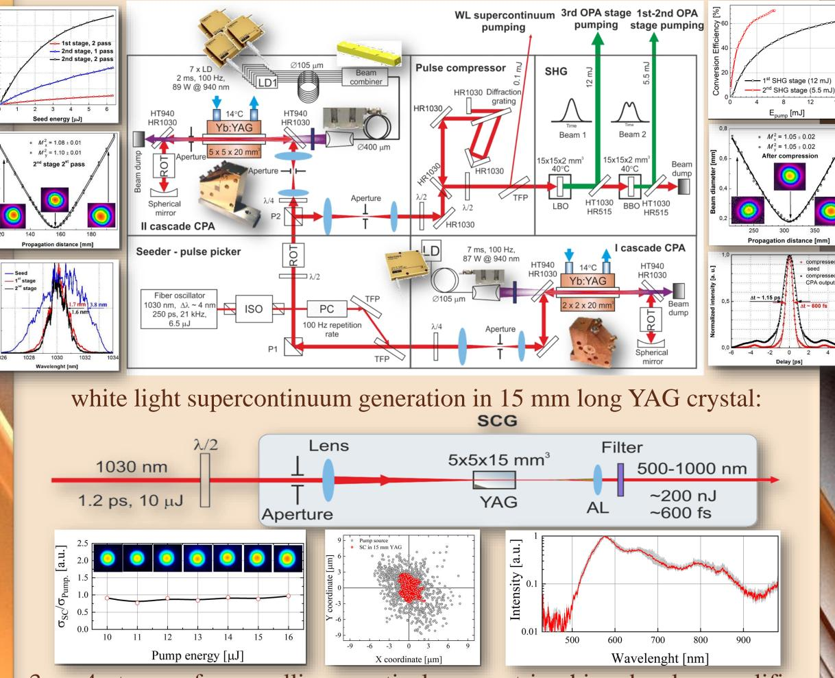
3 or 4 stages of non-collinear optical parametric chirped pulse amplifier (NOPCPA), and chirped mirrors (- 100 fs<sup>2</sup> GDD per bounce) compressor:
