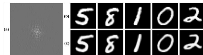
Figure 1. (a) The zoomed portion of a representative hologram, showing the interference fringes.
